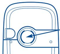
In handsfree mode, the speaker on the back of the phone is automatically activated. This speaker has a Hi-Fi membrane
