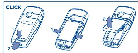
Unclip the battery and remove it.
